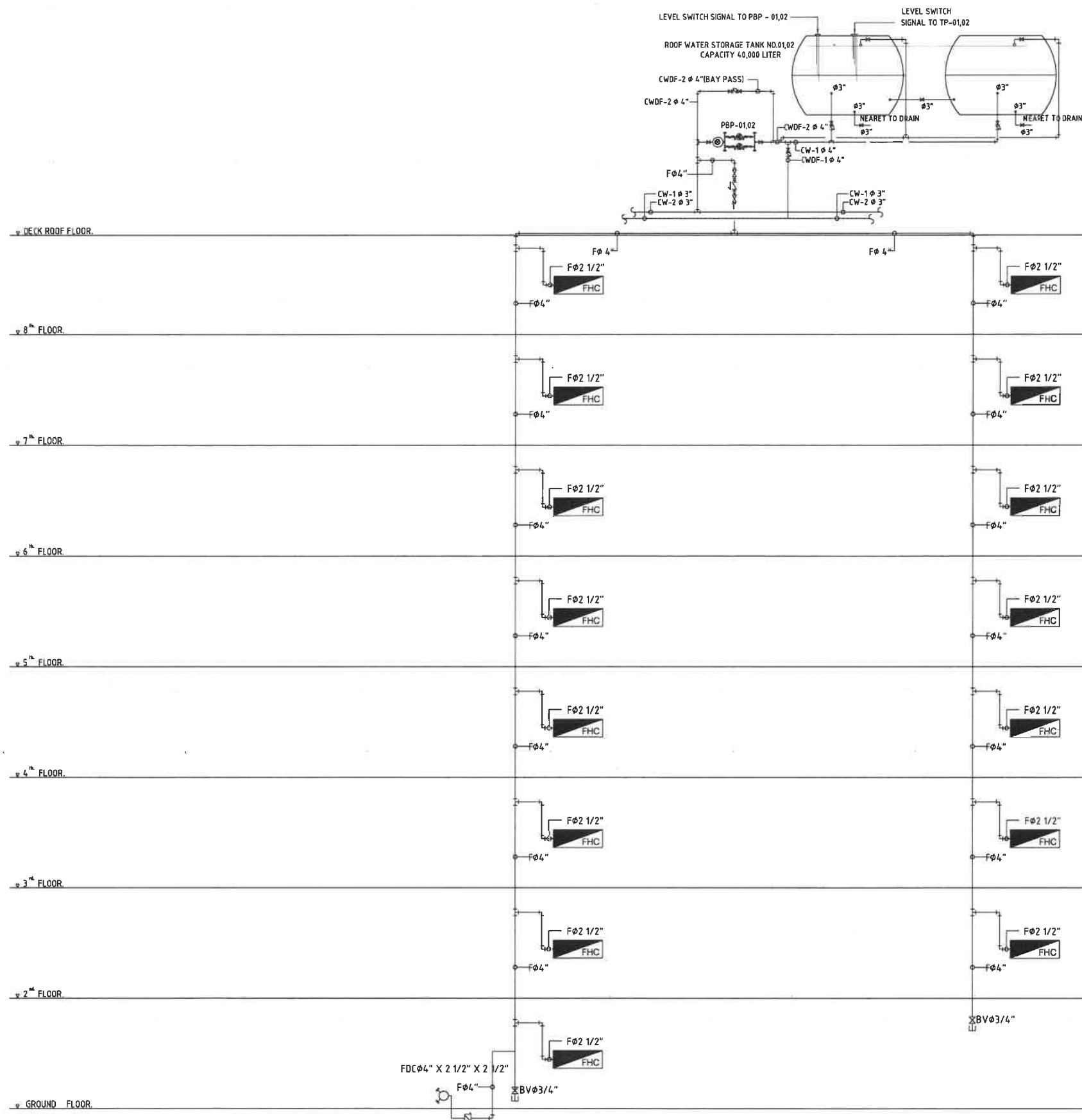
FIRE PROTECTION RISER
